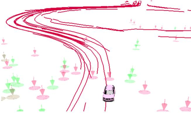
Fig. 4. Detected objects and their trajectories in a roundabout [13]. Dynamic objects are shown in red, static objects are shown in green, and unknown objects are shown in gray. The filtered trajectories of objects that are candidates for being vehicles are shown in red.
