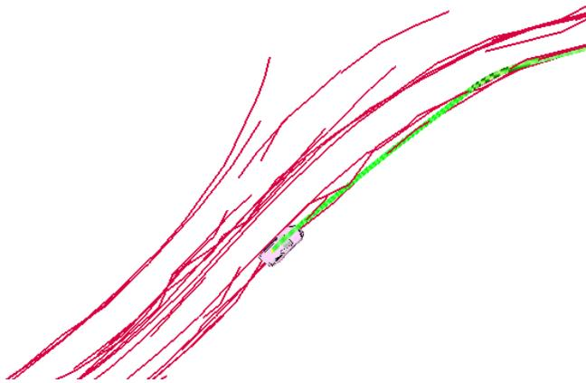
Fig. 7. Pathplanning with a temporary local map [13]. The generated trajectory is shown in green, the underlying trajectories are shown in red.
